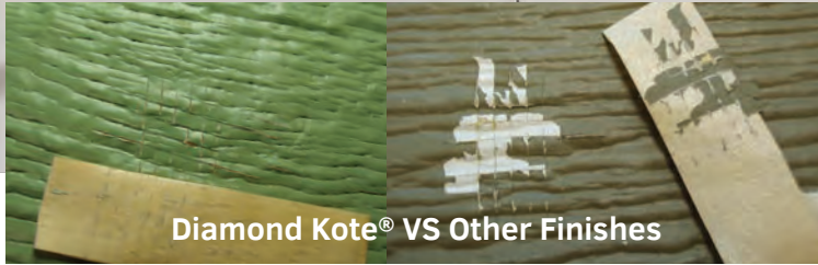
ASTM TEST D3359-09 - STRENGTH OF BOND
